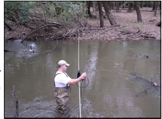
ANRA staff performs in-stream flow measurements on the Angelina River near SH 204.
