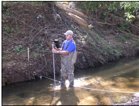
ANRA staff collect in-stream flow measurements using a Flow Tracker Handheld Acoustic Doppler Velocimeter (ADV).
