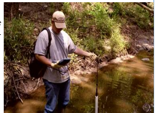
Water quality "Multiprobe" used for 24 hour measurements as well as routine water testing
