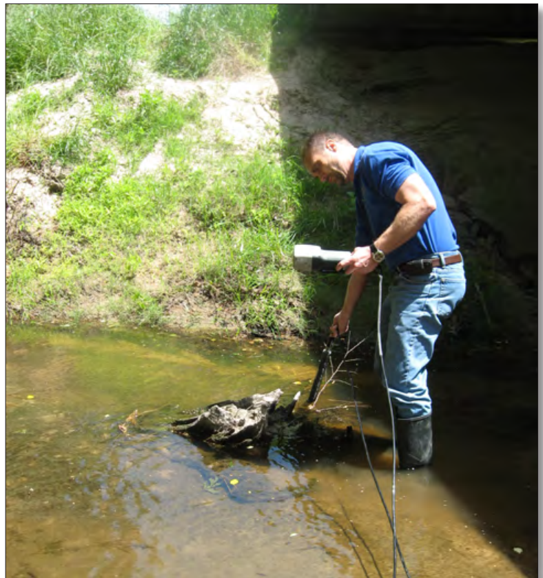
Measurement of pH, DO, Specific Conductance, and Temperature using a multiprobe instrument
