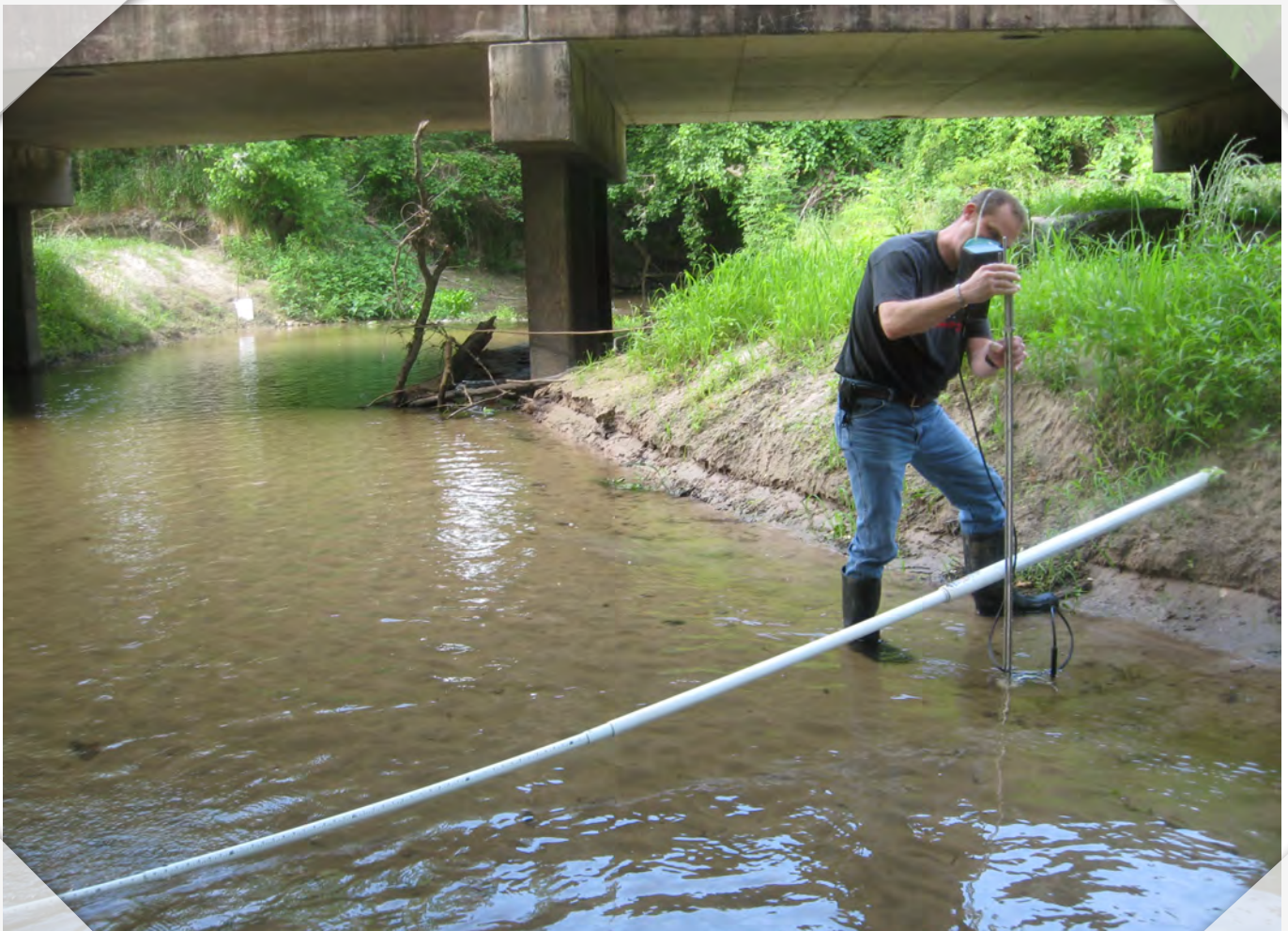
FLOW MEASUREMENT AT CEDAR CREEK AT FM 2497
